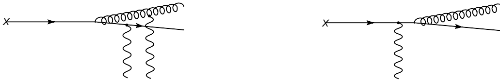
Figure 1: Illustration of QCD coherence. The emission of a soft wide-angle gluon receives contributions from Feynman diagrams in which it is attached to any of the external partons (left). The coherent sum of these diagrams is equal to the emission from a single parton with the total momentum and colour of the partons. That is, as if it were emitted before the smaller-angle harder gluon (right).
