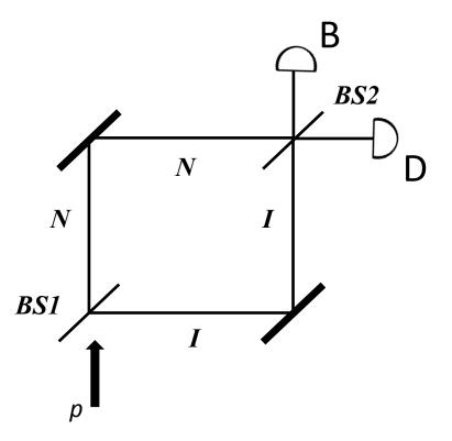
Figure 2. Schematic illustration of a single Mach-Zehnder interferometer. (See text to figure 1 for explanation of the symbols.) The beam-splitter BS1 is assumed to be a perfect, 50-50 beam-splitter, while BS2 is of a more general type (see text, in particular eq (14)).
